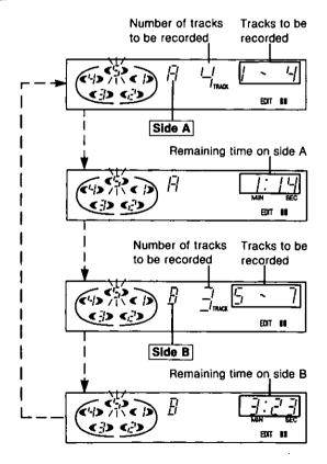
In this example, disc 5 can be recorded with tracks 1-4 on side A and tracks 5-7 on side B of the cassette tape.
